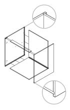
Bottom Panel inserted into the side panels. Reinforced with Stainless Steel Screws and Epoxy Adhesive
